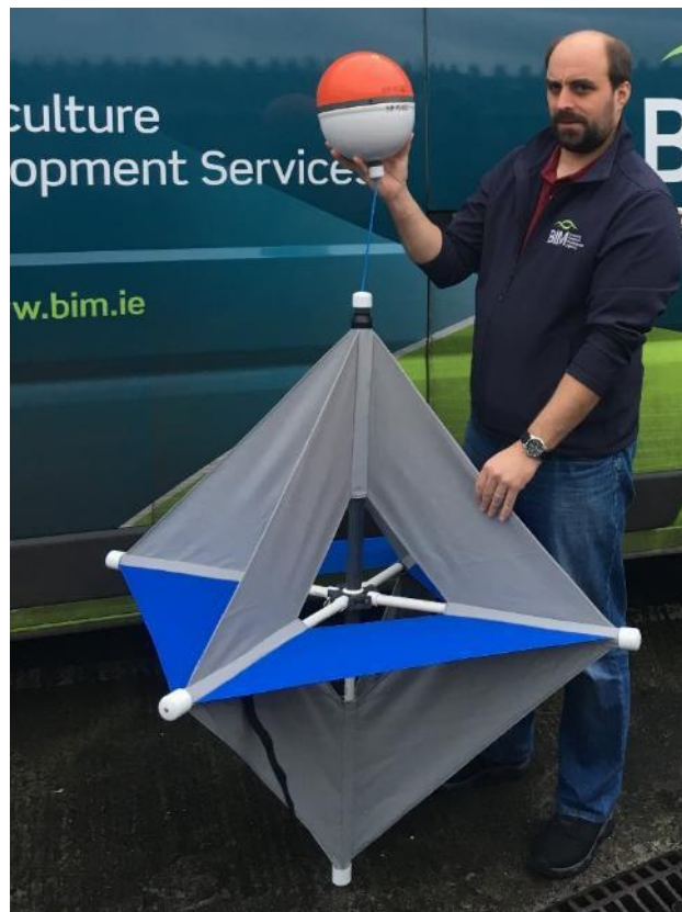
Figure 19: Detail of the Microstar GPS drifter
