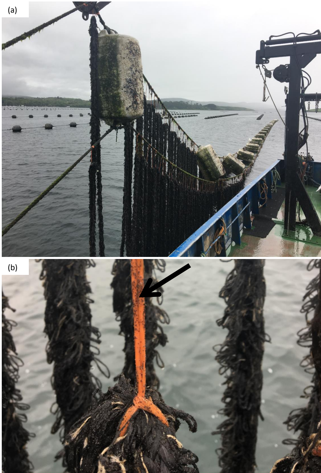
Figure 3: (a) ISPP test line raised for inspection. (b) Dense Mytilus spp. seed settlement above the rope (arrow).
